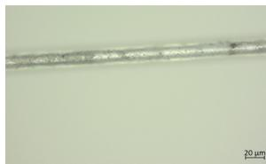
Abb. 78 Kristalline Ausblühungen (DM02\_OM01\_20x\_AL-POL\_20180301)
