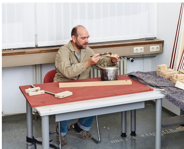
Fig. A7.2 Gluing wooden pipes
