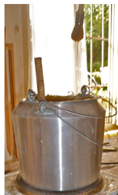
Fig. A7.3 Testing the fluidity of hide glue
