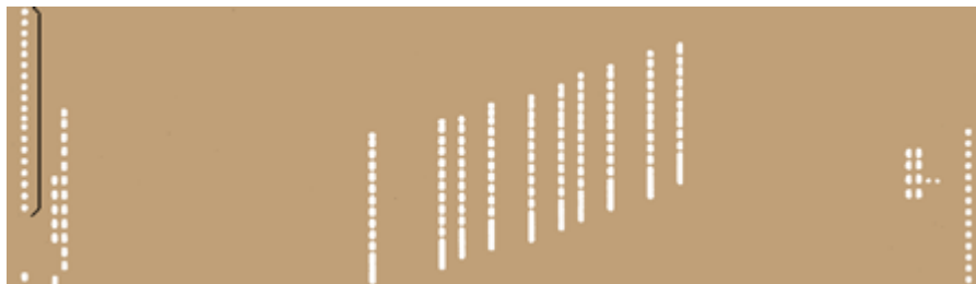
Fig. 9 Duo-Art roll with irregular row spacing. The punches in the sustain pedal track on the left should all be equally spaced. Similarly, the bridges in the note fields should all be of an equal size.
