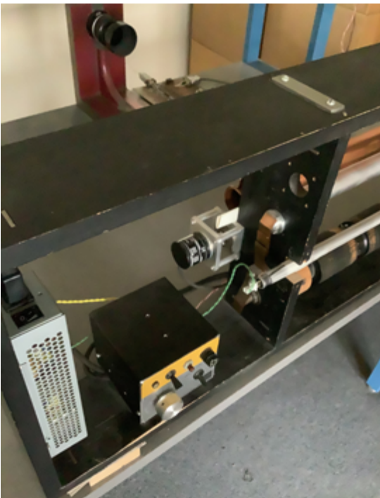
Fig. 5 The whole scanner with the left side of the roll transport in the front and the camera in the background.
