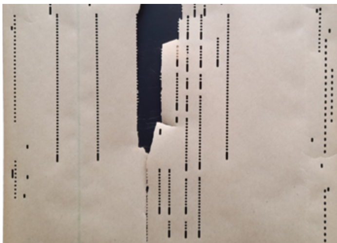
Fig. 1 This roll has become so brittle that it is now fast disintegrating.
