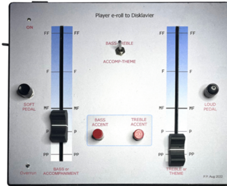
Fig. 13 Devised by Peter Phillips, this interface accepts a MIDI file of a player piano roll and has user-operated controls to add expression to the file when it is played on a MIDI piano, such as a Disklavier.
