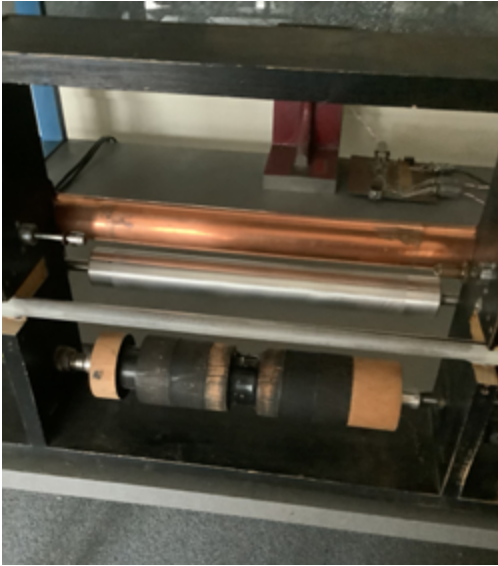
Fig. 6 Head-on view of the centre of the roll transport. Here, one can see the chucks for holding the roll, the copper-coloured tensioning bar, the aluminium measuring roller (125 mm in circumference) and the wooden take-up spool.
