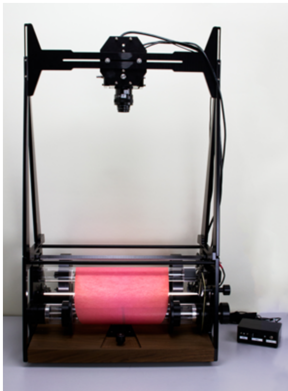
Fig. 1 Roll scanner used by Stanford University. The scanner has a camera that takes a series of photos as the roll is fed past the camera. The result is an image file of the entire roll. A MIDI file is generated from the image by software.
