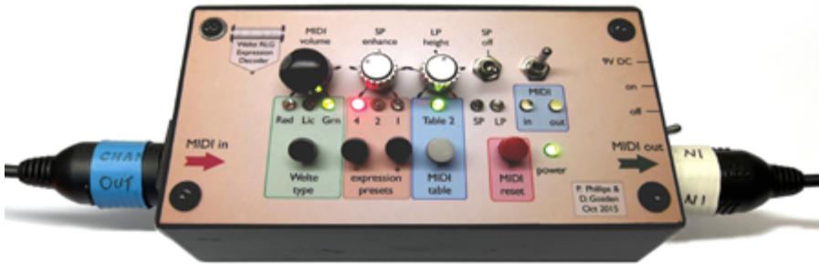
Fig. 6 An in-line Welte emulator. The input is an e-roll MIDI file and the output MIDI signal is the emulated version of the e-roll file. This is used in conjunction with a MIDI editor when working on a Welte e-roll MIDI file. The output of the emulator connects to a MIDI piano, such as a Disklavier.
