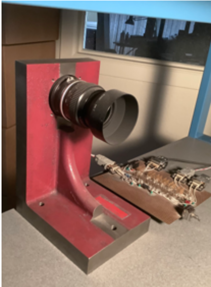
Fig. 3 The front of the camera. The lens and lens hood are clearly visible, as is the hand-made circuit board on the table.
