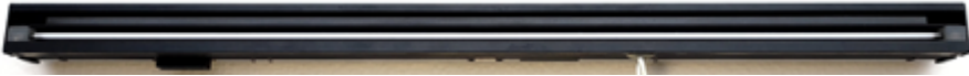
Fig. 4 A contact image sensor. The white cold cathode fluorescent lamp (CCFL) and the rod lens are mounted within separate channels so that no direct light passes between them. A row of image sensors is mounted inside the sealed unit behind the rod lens.
