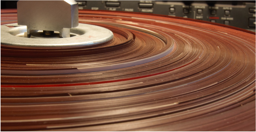
Fig. 1 A typical magnetic tape of the Oskar Sala Collection: loose, stepped wrapping, countless cuts and glue areas.
