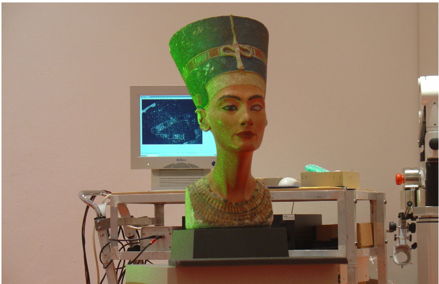
Fig. 6 Video holography, acoustically induced diagnosis of plaster detachments, on the bust of Queen Nefertiti, National Museums Berlin 2009, with physicists from Carl von Ossietzky Universität, Oldenburg.
