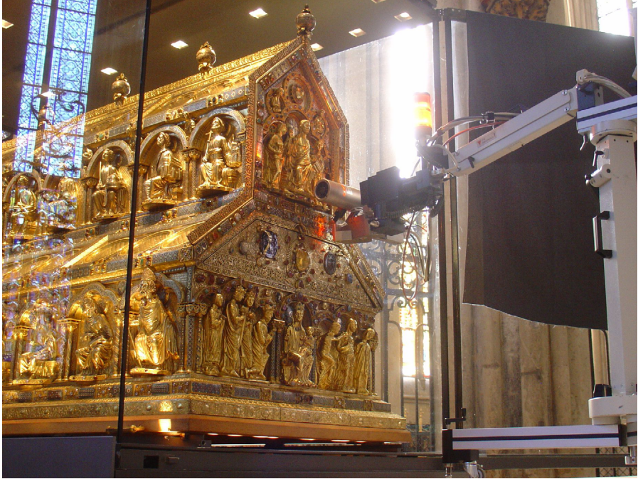
Fig. 5 \mu -XRF investigation on the enamels of the Shrine of the Three Kings, completed by Nicholas of Verdun ca. 1225, Cologne Cathedral, 2007.
