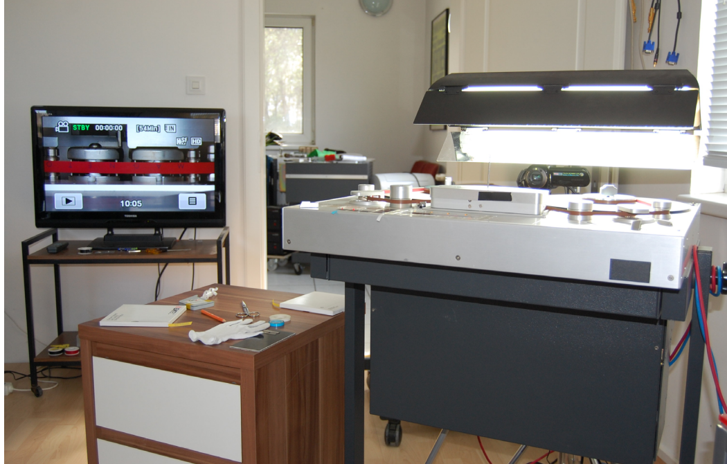
Fig. 9 The setup for recording and digitising the tapes.
