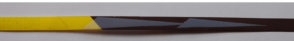
Fig. 8 Wedge-shaped cut pieces of adhesive tape attached to the layer side to achieve special effects.
