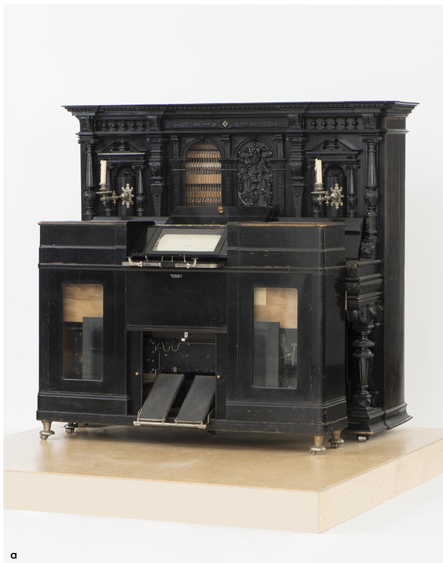
Fig. 1a–d Push-up player (in front of a regular piano), Phonola, Hupfeld, c. 1905, Deutsches Museum Munich # 31069.
