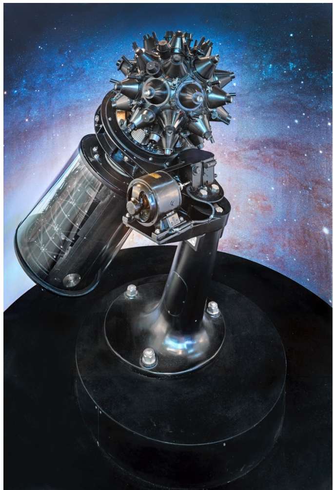
The first star projector: the Zeiss Modell I in the Deutsches Museum.
