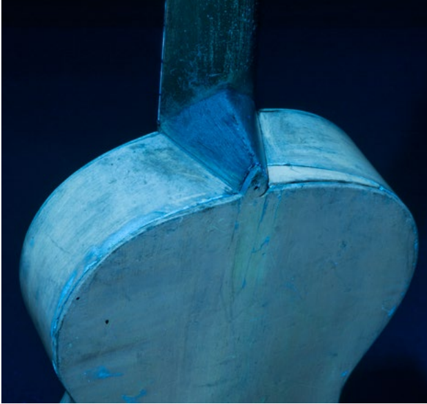
Figure 32 Detail of the neck heel and the back of DMO 5430 during its examination under ultraviolet light.
