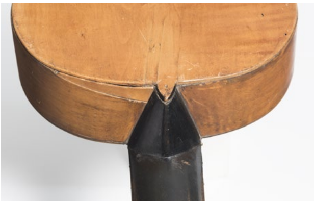
Figure 19 Detail of the neck-heel join of DMO 5430 showing the thin, wedge-shaped piece of maple glued on the bass side.
