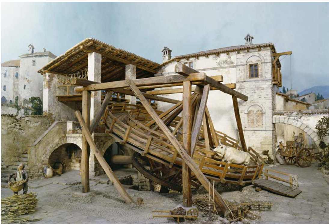
Figure 20 A timeless and unique diorama – “Ox on a treadmill,” a historical example of power machinery in the exhibition Power Engines.
